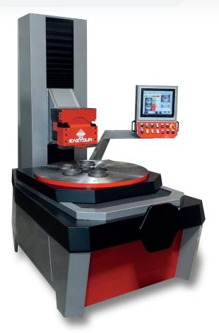
Integral Rotary was designed by Easydur as a **production hardness tester**. It can be considered a working island, as it is equipped with a test axis and an additional turning table, as well as a second Y axis to move the turning table back and forth in relation to the head.
