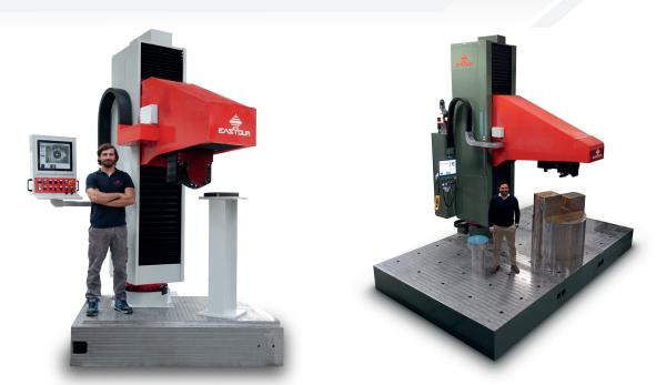
EASYFLAG 3000 is a flag hardness tester for Brinell tests specifically designed for testing **medium and large forged items**.
