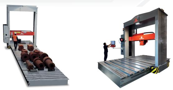
EASY 3000 is a portal hardness tester for Brinell and Rockwell tests specifically designed for testing medium, large and very large forged items.
