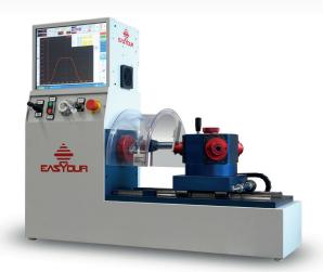
This torque meter has a touch screen computer for running test recipes. Freestanding and self-bearing models are available.
