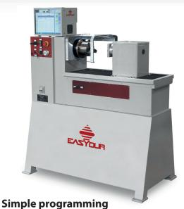
This torque meter has a touch screen computer for running test recipes. Freestanding and self-bearing models are available.
